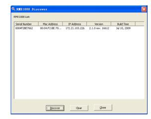
**4** Run the Web browser on the PC. Enter http://<RMX 1000 IP address> in the address bar, and then press Enter.
